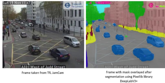
Fig. 5: A TfL JamCam frame with and without the Pixellib segmentation mask
