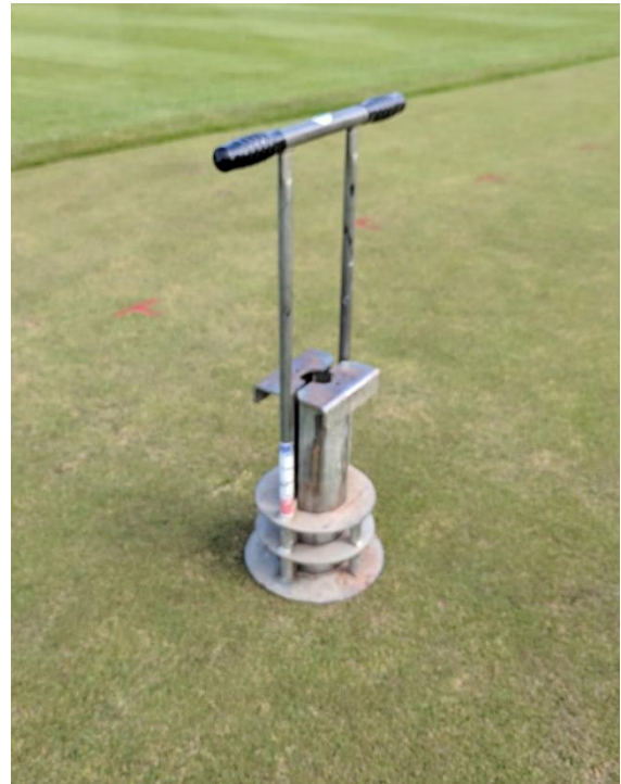
Figure 65: A hole changer used in golf courses to swap holes on a green.
