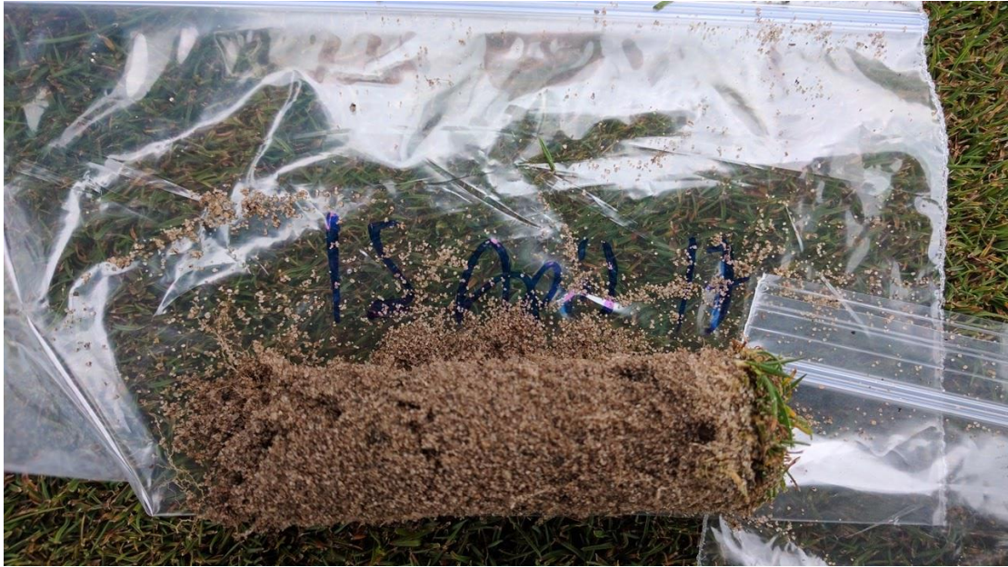
Figure 5: A 2.5cm diameter soil core and the sandwich bag it was stored in.
