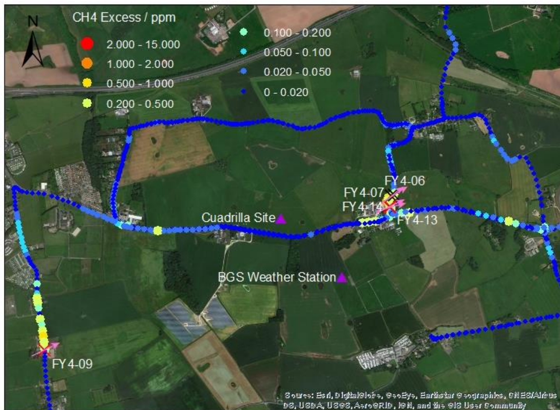
Figure 12: Methane excess recorded in the vicinity of the Cuadrilla site on (a) 24/10/17 (top) and (b) 25/10/17 (bottom).
