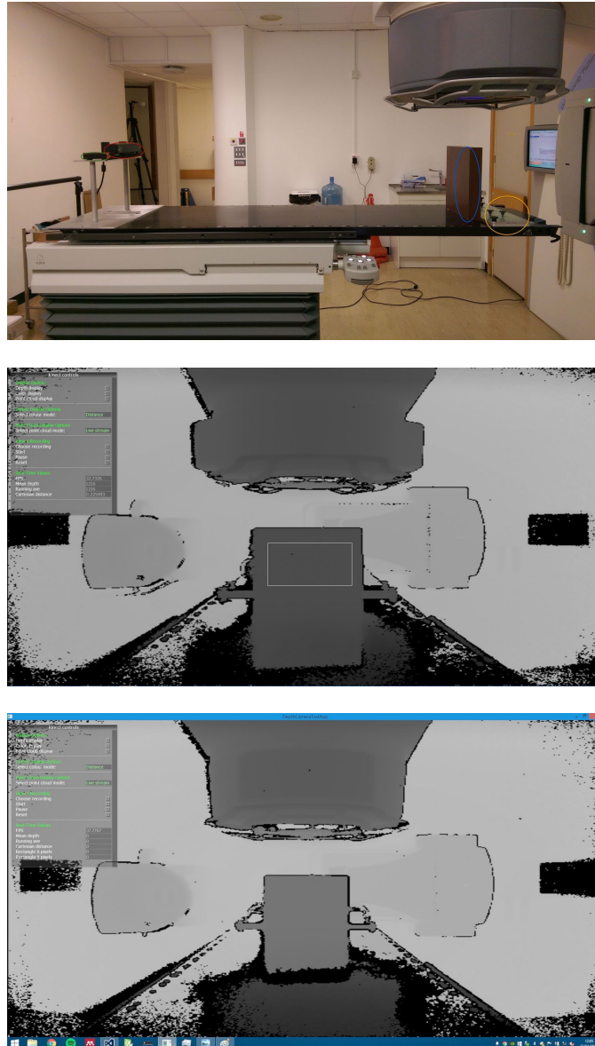
FIG. 1. Experimental setup and effect of electromagnetic interference on the displayed images. (Upper panel) The sensor (red) is mounted on a custom stand manufactured in-house. A thermometer is attached to the upper exhaust vent on the sensor. The Leica Disto D210 laser measure (green) is mounted securely next to the sensor, with the front plane lined up with the sensor. To the right, the solid water phantom (blue), used as the target, can be seen, along with the metal cross-plate (orange) screwed into the couch which ensures the phantom is perpendicular to the sensor. (Middle panel) A depth camera view of a linac and solid water phantom on the treatment couch; darker objects are closer to the camera and lighter objects are further away. A region of interest (ROI) drawn by the user on the phantom is shown as a gray outline. The mean Kinect reported distance value of the pixels in this (ROI) in every frame was recorded to a file. Image was taken without the PFN operating. (Lower panel) Worse-case image, with a PRF of 400 Hz. The circled region on the image indicates a region where additional image artifacts were observed.
