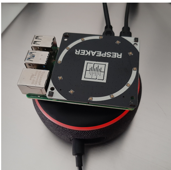
FIGURE 7.4: Placement of Echo Dot and Respeaker 4-Mic Microphone Array During the Recording of The Dataset
