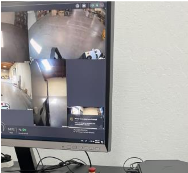
Figure 144 Popup message occluding the fork camera (bottom right of the screen)
