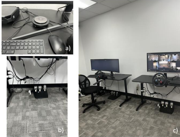
a) key board and mouse with audio microphone b) foot pedal (clutch, accelerator, brake (left to right) c) remote operator work station curved (left) and flat screen (right) n.b., note relative height of monitors and position of steering wheel
