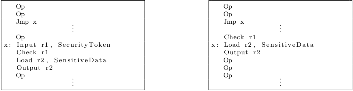
Figure 5.3: When protected by only simple hardware-software binding, the code snippet on the left can be modified to leak sensitive data by moving code into a location reached by a JUMP operation.
