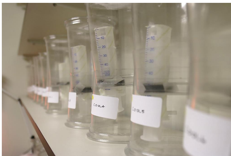
Figure 2.4 Modular plastic cages used for clothianidin dosing of workers (Chapter 7) developed by Heard & Hesketh (2017).
