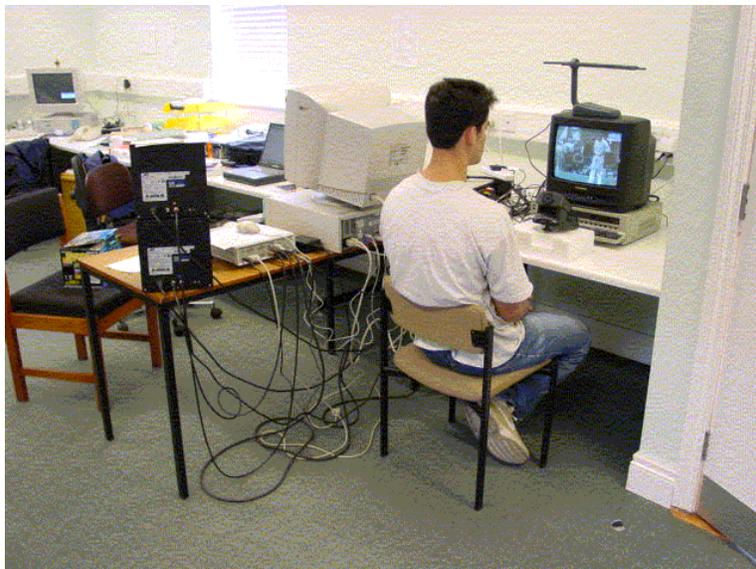
Figure 2. Eye is tracked using an ASL 504 Tilt/Pan infra red camera which is connected to a host computer through a control box. Video signal and eye trace data are combined into another workstation (partially obscured by the computer monitor) for processing.
