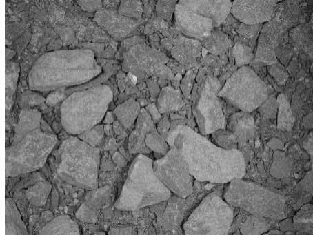
Figure 1: An image of construction aggregate. The properties of the aggregate are defined by size for larger pieces, and by granularity for finer pieces.
