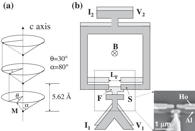
FIG. 1. (a) Magnetic structure of Ho: Magnetization  $M$  rotates by  $30^\circ$  each atomic layer along the  $c$  axis at an angle of  $80^\circ$  to this axis. (b) Experimental setup and SEM micrograph of the  $S/F/S$  junction area prepared by shadow evaporation. Sample with  $L_F = 120$  nm.
