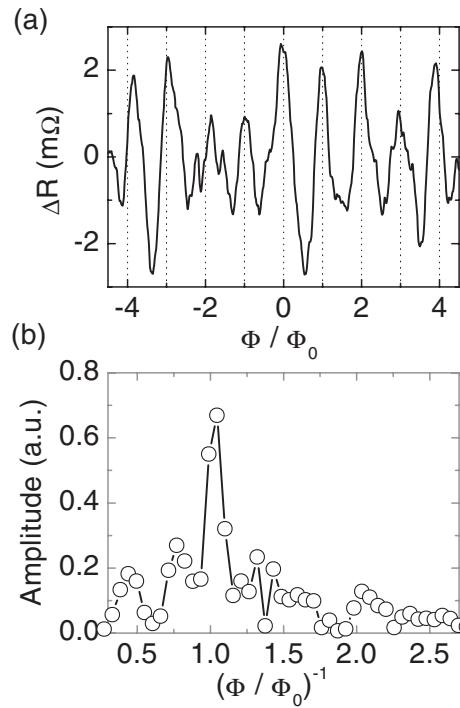
FIG. 3. (a) Magnetoresistance oscillations of the sample shown in Fig. 1(b) measured at  $T = 0.27 \text{ K}$  as a function of a normalized external flux through the loop. Sample resistance is  $94.3 \Omega$ .  $L_F = 120 \text{ nm}$ . (b) Fourier spectrum of the oscillations confirming the  $hc/2e$  periodicity.
