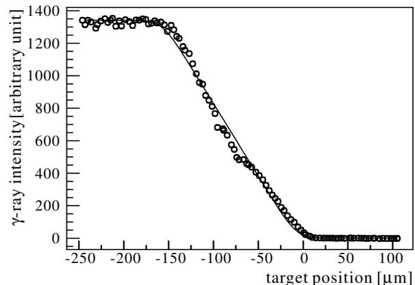
FIG. 3. The  $\gamma$  ray intensity as a function of the target position (open circles). The  $\gamma$  ray intensity was corrected by the beam intensity. The solid curve is the result of the fit to Eq. (4). See text.
