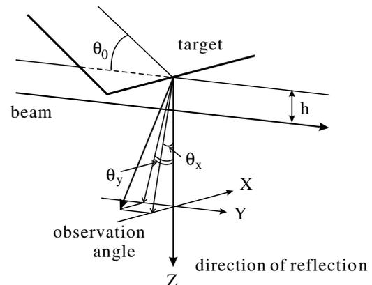
FIG. 1. Geometry of DR near a semi-infinite target.
