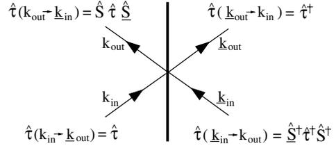
FIG. 1. Scattering geometry illustrating the scattering channels and the corresponding transfer amplitudes for the model discussed in the text.
