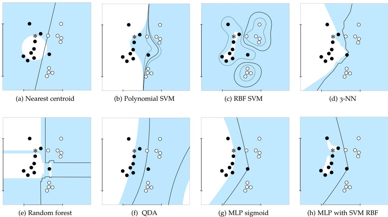
Figure 6.1: Possible NCMs for different classifiers. The solid line depicts the decision boundary between classes ● and ○, the dotted lines show SVM margins. Shaded areas capture points which are *more nonconform* (i.e., ‘less similar’) than the new test point (\*), with respect to class ●.
