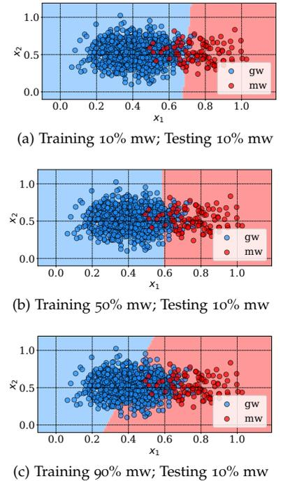
Figure 5.3: Example of training bias with Linear-SVM and two features. Test set is fixed at 10% malware but as rate in the training set increases, the decision boundary moves towards goodwill, improving Recall but decreasing Precision.
