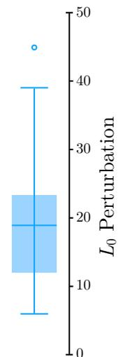
Figure 4.8: Distribution of  $L_0$  norm perturbations (*i.e.*, number of binary features added) induced by the most effective individual transformations (UER  $\geq$  90%).
