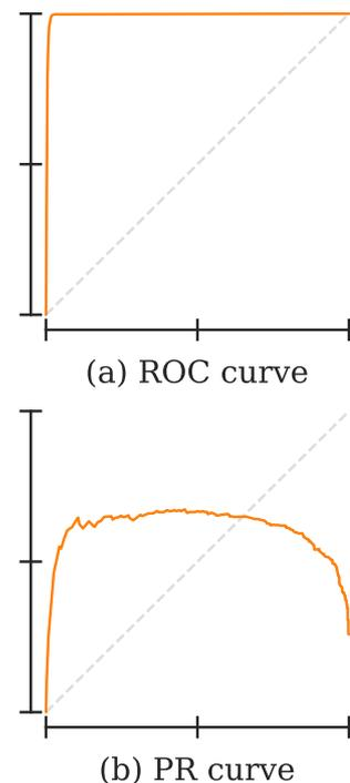
Figure 5.14: ROC and PR curves applied to results on an artificial dataset with an imbalanced class ratio. While the classifier's decision scores are the same in both cases, only the PR curve conveys the true performance.
