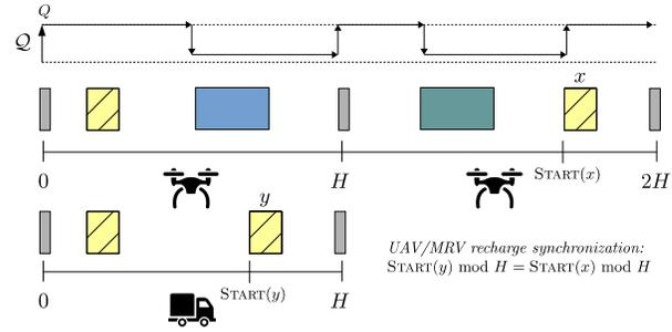
Fig. 2. CP model, single resource transformation technique. Two UAVs,  $|O| = 2$ , with augmented horizon ( $2H$ ). Single MRV,  $|K| = 1$ . Each UAV conducts one search pattern (blue/green) and is recharged once (yellow) by the MRV.
