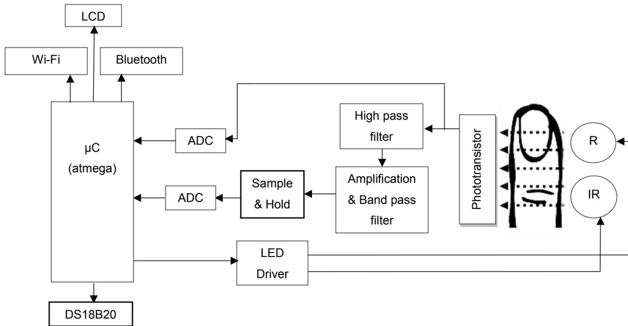
Fig. 5 Health Monitoring Block Diagram
