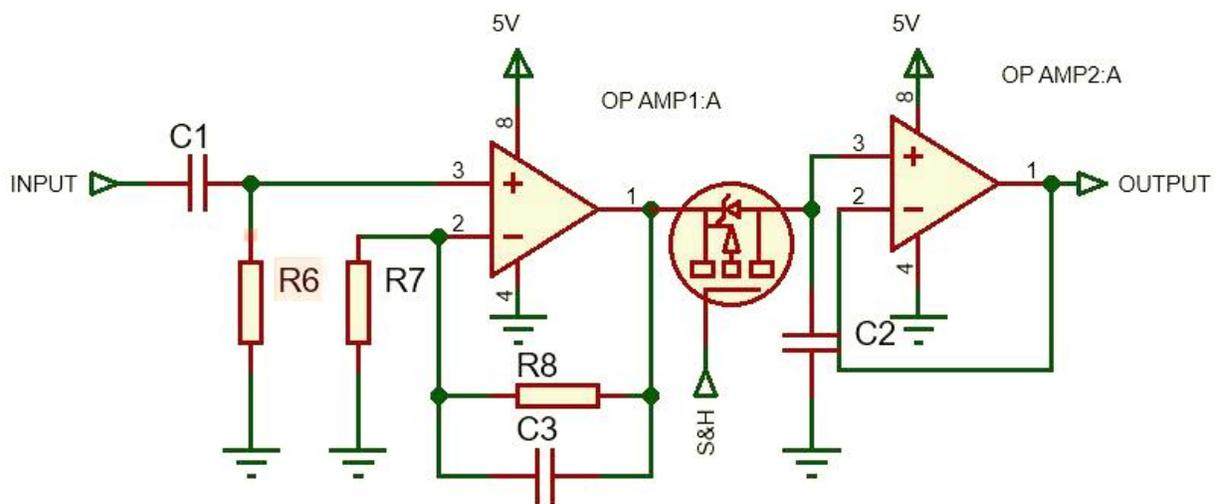
Fig. 3 Conditioning & Sample/ Hold Circuit
