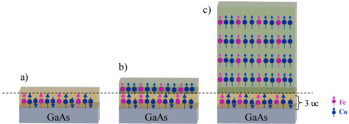
FIG. 4. Schematic diagrams of  $\text{Co}_2\text{FeAl}$  thin films with thicknesses of (a) 3 uc, (b) 5 uc and (c) 20 uc. Yellow area exhibits the interfacial layer with weak magnetization. Green area represents bulk-like ferromagnetic layer.
