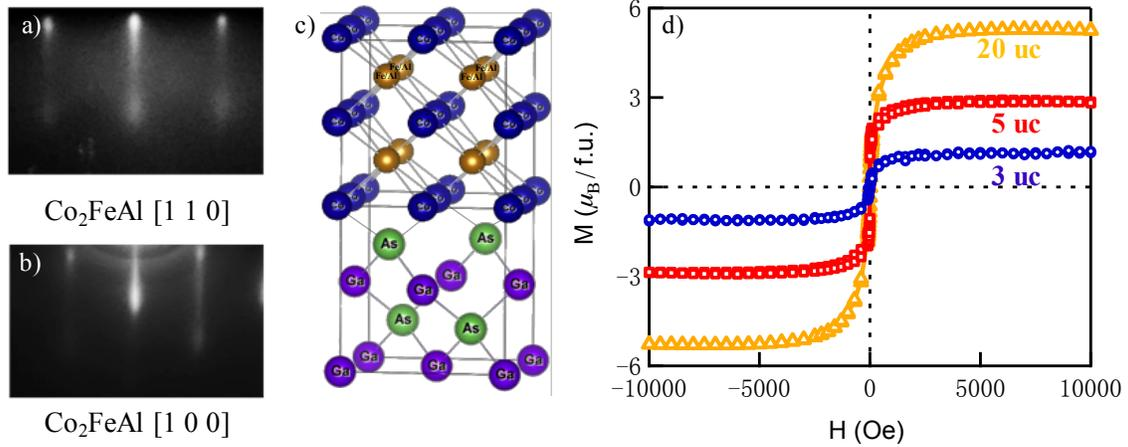
FIG. 1. RHEED and VSM measurements. RHEED patterns of (a)-(b) grown  $\text{Co}_2\text{FeAl}(001)$  film with an electron beam along  $[110]$  &  $[100]$ , respectively. (c) Schematic view of  $\text{Co}_2\text{FeAl}/\text{GaAs}(001)$  heterostructure. (d) Magnetization of  $\text{Co}_2\text{FeAl}$  films with thickness of 3 uc, 5 uc and 20 uc measured in plane at 300 K.
