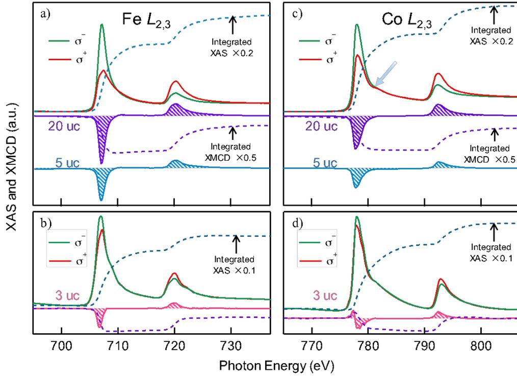
FIG. 3. XAS and XMCD measurements. Typical pairs of XAS and XMCD spectra of (a)-(b) Fe and (c)-(d) Co for Co<sub>2</sub>FeAl films with thickness of 20 uc, 5 uc and 3 uc grown on GaAs(001) measured at 300 K.  $\sigma^+$  and  $\sigma^-$  stand for the XAS probed by left and right X-ray helicities, respectively. The dashed lines represent the integrations of the spectra.
