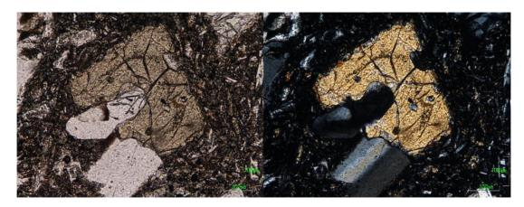
Figure 3-1 Olivine in GU1 showing evidence of resorbed edges and embayments. PPL is shown on the left hand side and XPL on the right.
