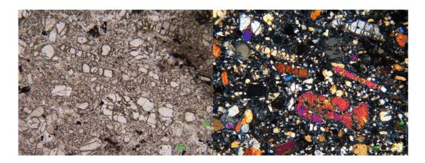
Figure 3-4 Skeletal and elongate olivines in CA3. The olivines also show chlorite alteration along cracks in the crystals.
