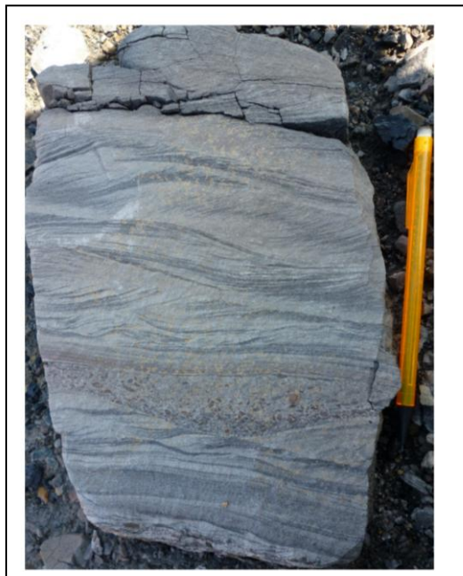
FIG. 3.11 Field photograph of climbing ripples on a loose block of siltstone from the interseam sediments overlying seam 92. The surface of the block is perpendicular to bedding and a microchannel and different types of ripples including climbing ripples are observed. Scale bar = 15cm.
