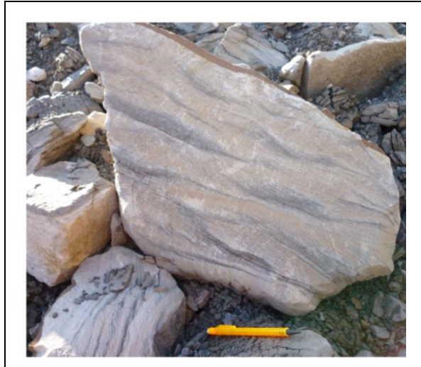
FIG. 3.10 Field photograph of climbing ripples on a loose block of fine-grained sandstone/ siltstone from the interseam sediments overlying seam 91 (Mine 2). The surface of the block (with ripples) is perpendicular to bedding. Scale bar = 15cm.
