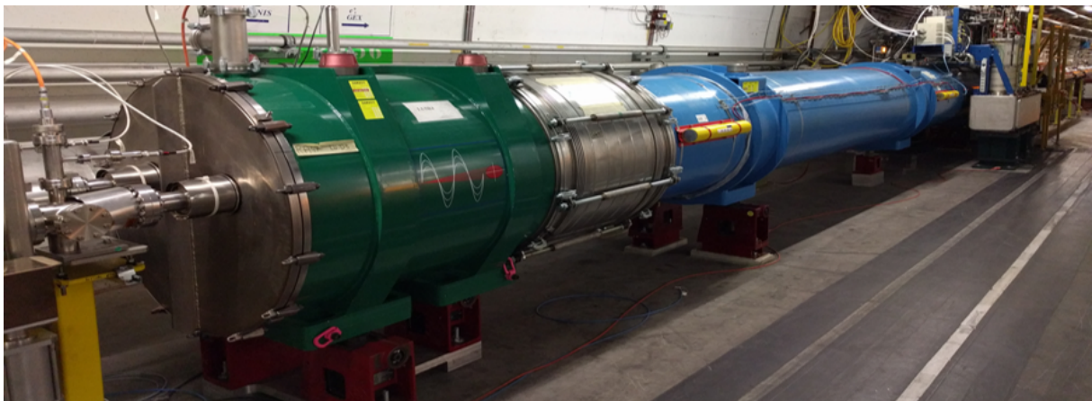
Figure 3.1: Schematic diagram (a) illustrating the layout of the synchrotron radiation source used for beam diagnostics at the LHC. The vertical scale is exaggerated to emphasize the beam deflections within the magnetic devices. The extraction system is shown for Beam 1 only. In (b), a picture of the superconducting undulator (green) and the D3 dipole (blue) installed on the right-hand side of the long straight section located at Point 4.
