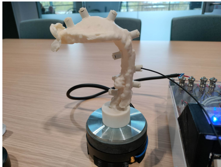
Figure 6.3: Photograph of 3D printed vocal tract model with microphone guides and plugs fitted. The microphone is currently inserted into a guide on the right side of the image.
