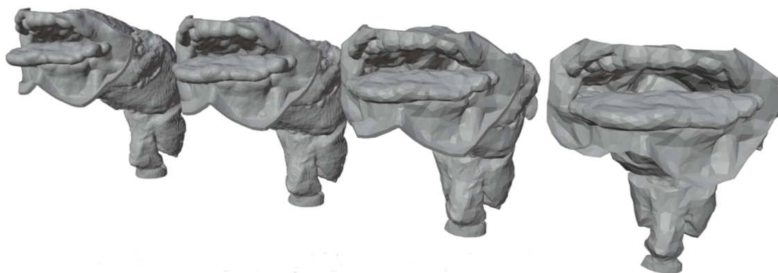
Figure 4.2: Vocal tract model of Nesyamun ‘True of Voice’ with decreasing number of vertices from 500 000 on the left to 3000 on the right.
