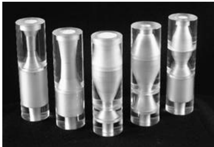
Figure 4.17: The five Arai vowel sound cylinders (from left: /i/, /e/, /a/, /o/, and /u/) [11].
