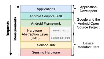
Figure 1: Components, corresponding owners, and information flow of the Android sensor stack (adapted from [8]).
