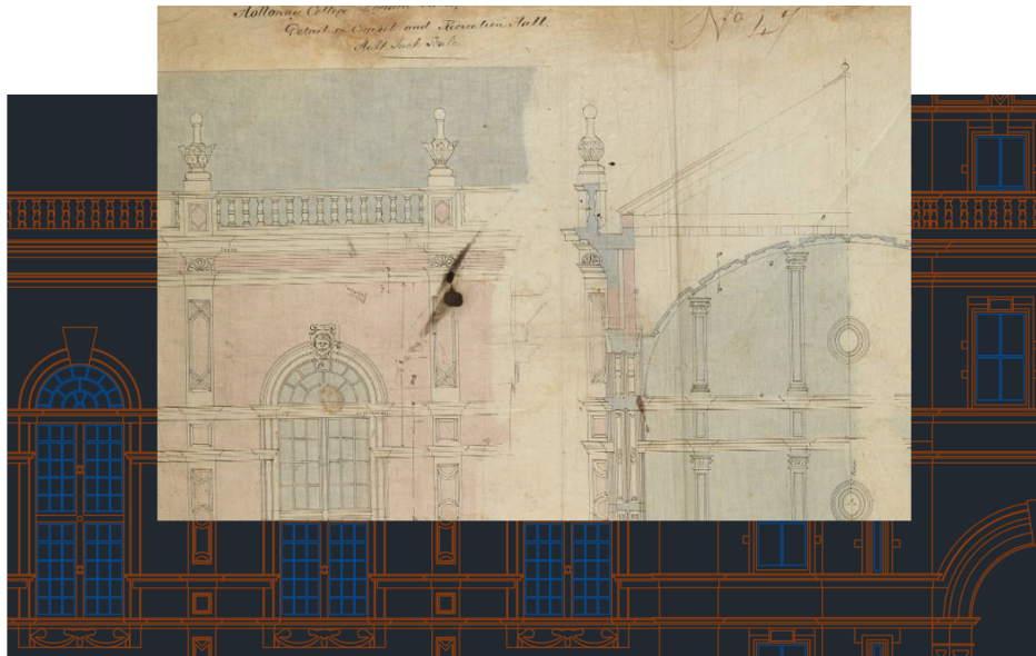
Figure 4.3: A side by side comparison of a CAD drawing of the chapel with one of the original architectural drawings. This was utilised to find the radius of the arched ceiling.
