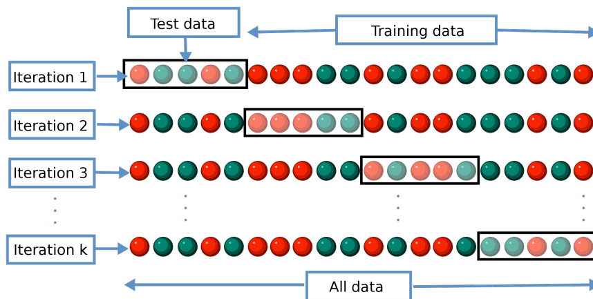
Figure 10.20 A conceptual illustration of the method known as k -fold cross-validation, by which the performance is assessed as an average across k iterations. The data is split into k subsets known as folds, and for each iteration one of these folds is held back to assess the performance, while the other k - 1 folds are used for training [208].
