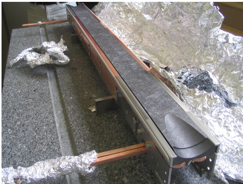
Figure 1.18: Graphite jaw of a LHC secondary collimator [38], the graphite jaw is 1 m long and features two tapered ends.
