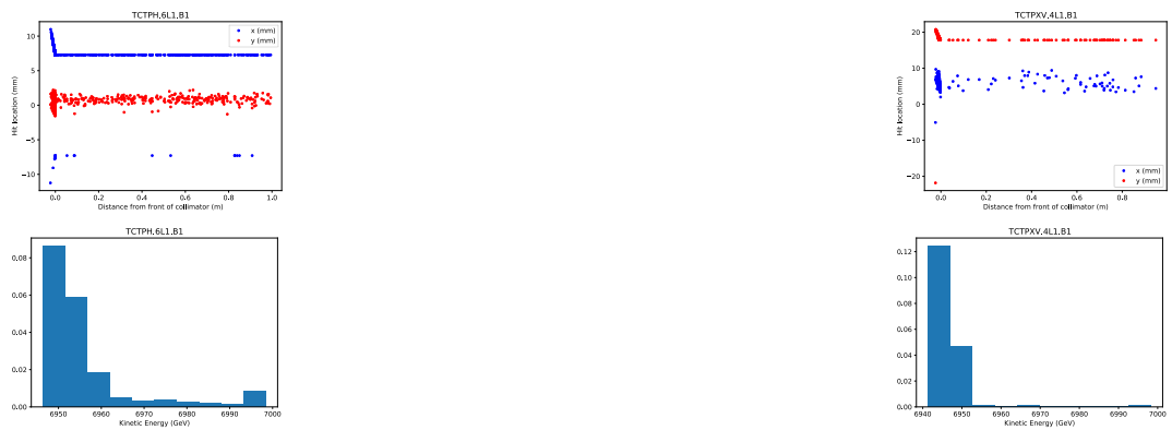
Figure A.10: Distribution of hits (top) and their kinetic energy (bottom) for TCTs for optics with \beta^* = 100 cm.
