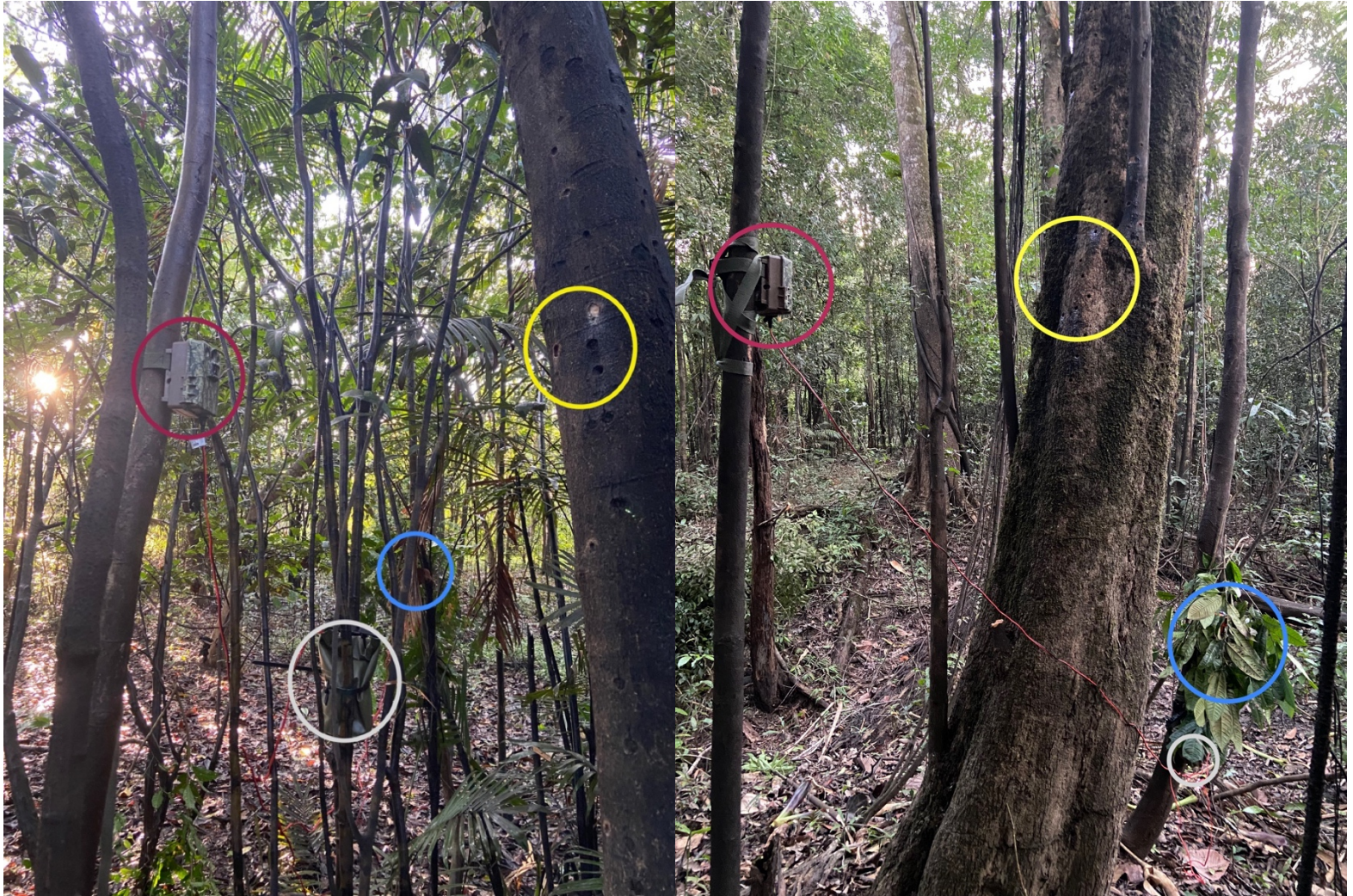
Figure 6.10 Experimental ABR setup. The maroon circle denotes the position of the camera trap, the grey circle the position of the battery pack, the blue circle the placement of the speaker and the yellow circle highlights the active sap holes. The image on the left was taken at the group TL14 and the right is the group RC2.
