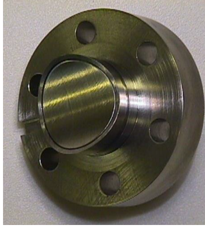
Figure 1.7: Button BPM pickup [16,18].
