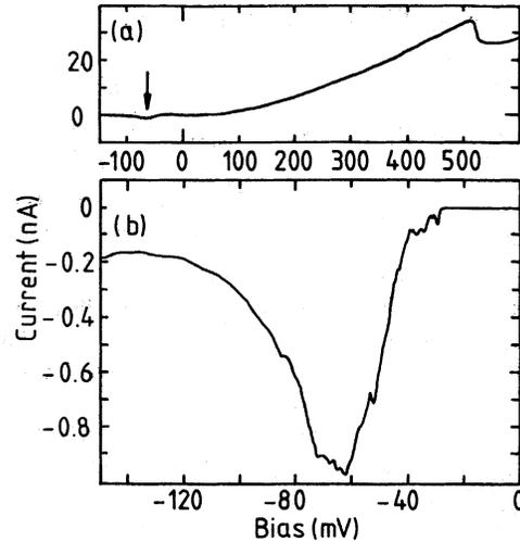
FIG. 2. (a) Current-voltage ( $I$ - $V$ ) characteristics of a 1- $\mu$ m-diam asymmetric GaAs-Al<sub>x</sub>Ga<sub>1-x</sub>As resonant tunneling diode. The strong asymmetry of the  $I$ - $V$  is due to charge accumulation in forward bias. The arrow indicates the small ground-state resonance in reverse bias. (b) Expansion of the reverse bias ground-state resonance, showing fine structure over the whole resonance peak.
