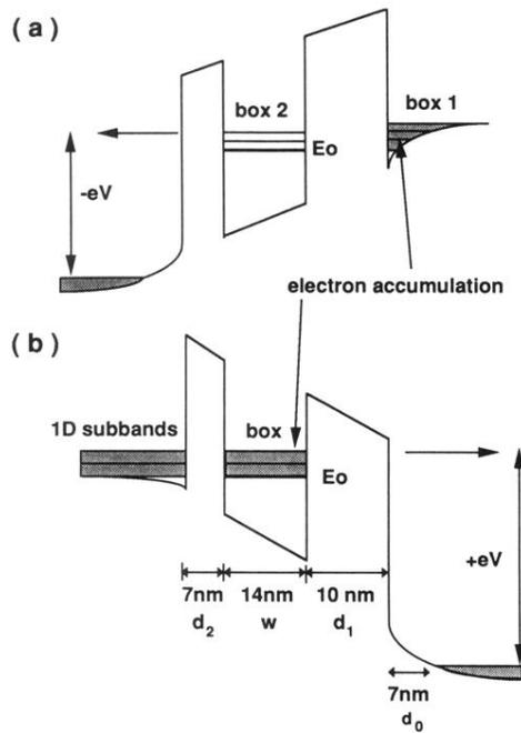
FIG. 1. Band diagram of the asymmetric GaAs-Al<sub>x</sub>Ga<sub>1-x</sub>As double-barrier structure, illustrating the tunneling mechanism. 1D subbands are formed in the contact regions, and 0D states are created in the well. (a) In reverse bias electrons tunnel from the 0D states in the accumulation layer (box 1) into the 0D states in the well (box 2). (b) In forward bias, electrons tunnel from the 1D subbands into the 0D states in the well.
