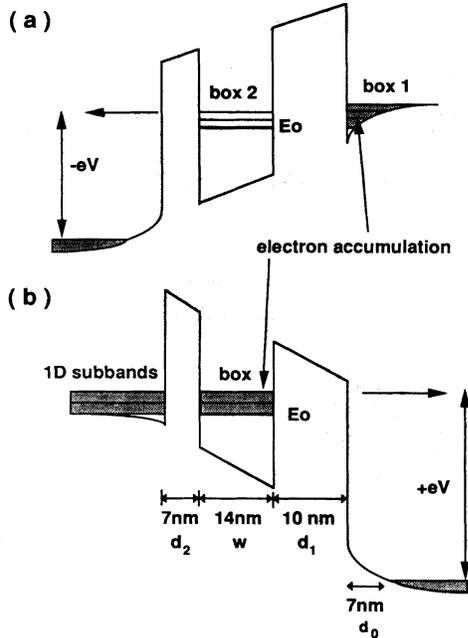
FIG. 1. Band diagram of the asymmetric GaAs-Al<sub>x</sub>Ga<sub>1-x</sub>As double-barrier structure, illustrating the tunneling mechanism. 1D subbands are formed in the contact regions, and 0D states are created in the well. (a) In reverse bias electrons tunnel from the 0D states in the accumulation layer (box 1) into the 0D states in the well (box 2). (b) In forward bias, electrons tunnel from the 1D subbands into the 0D states in the well.
