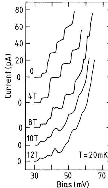
FIG. 4. Detailed  $I-V$  characteristics for low forward biases, as a function of a magnetic field applied parallel to the current.
