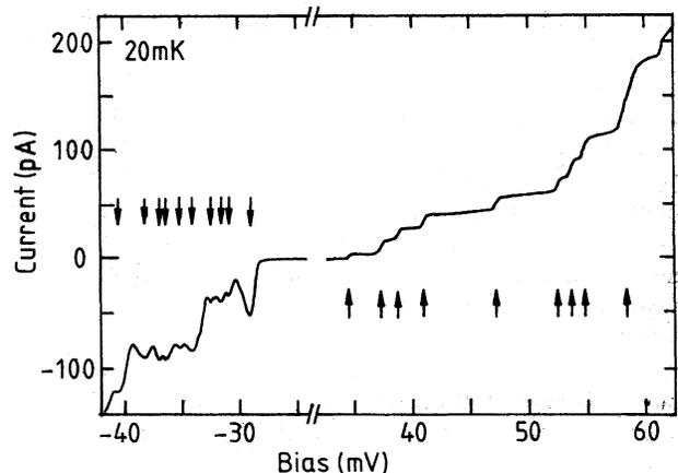
FIG. 3. Details of the  $I$ - $V$  characteristics in Fig. 2, showing the steps with large plateau widths in forward bias. In reverse bias the resonance spikes show tunneling between two quantum boxes in series (0D-0D tunneling) and the small spike spacing in bias is assigned to the single-electron spectrum without electron-correlation effects.
