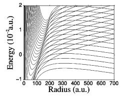
FIG. 4. Adiabatic eigenvalue curves for a hydrogen atom in parallel electric and magnetic fields of strengths 51.4 kV cm<sup>-1</sup> ( $1 \times 10^{-5}$  a.u.) and 470 T ( $1 \times 10^{-3}$  a.u.) respectively.
