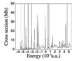
FIG. 6. The photoionization spectrum corresponding to the transition from the ground state to the m=0 final states of hydrogen in parallel electric and magnetic fields of field strengths F= 51.4 kV cm<sup>-1</sup> ( $f=1 \times 10^{-5}$  a.u.) and B=470 T ( $\beta=1$  $\times 10^{-3}$  a.u.), respectively. The dotted line represents the Stark saddle energy plus the first Landau threshold or zero-point energy.
