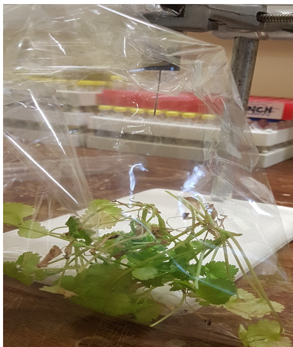
Figure 69: SPME probe absorbing gas emissions from inert plastic bag with harvested Coriander.
