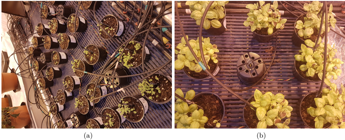
Figure 70: Non randomised layout for Gas sensor trials. Pots of the same treatment are orientated around each gas sensor in blocks. Gas sensor can be seen at approximate crop height on upturned pot.
