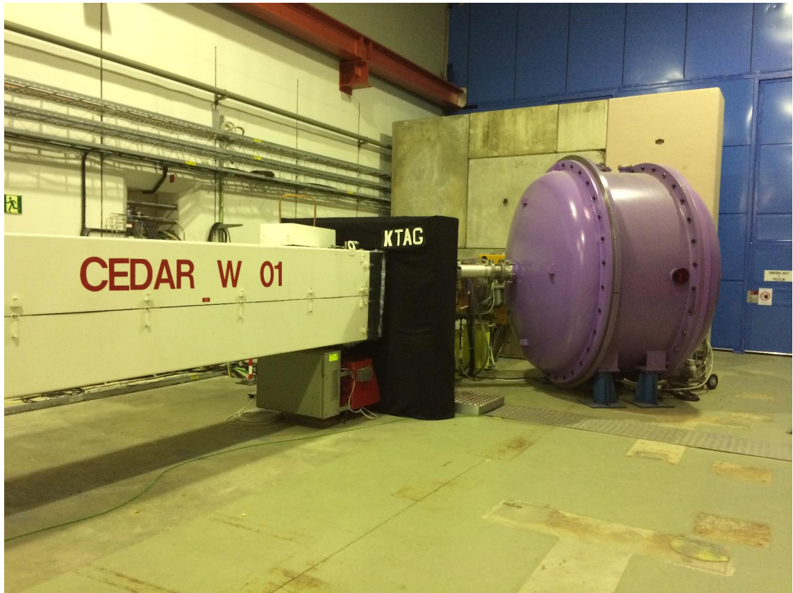
Figure 4.5: A photograph of the CEDAR (KTAG) detector located in the K12 beam line of the NA62 experiment [65].
