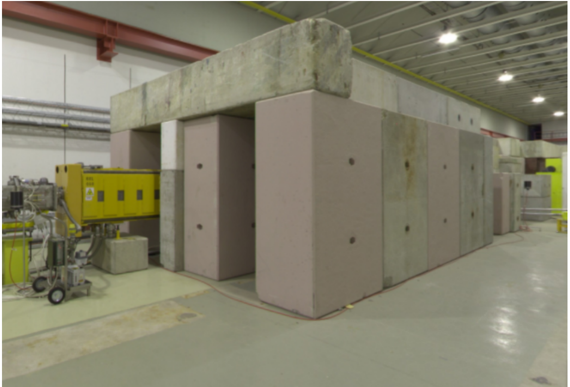
Figure 8.20: Shielding in the region after the first achromat in the current NA62 configuration.
