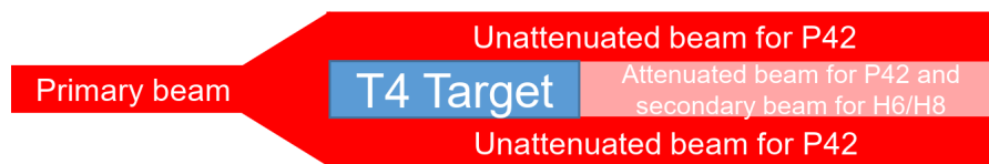
Figure 8.10: Schematic side view of proton beam being defocused before T4 target and partially interacting with it [118].
