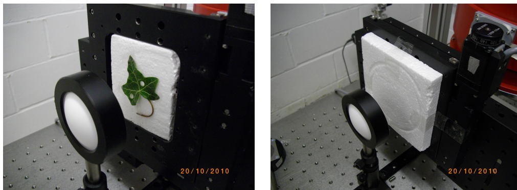
Figure 5.10: Left: Photograph of a leaf mounted onto a polystyrene slab, showing the position of the hole-punches. Right: The leaf during a scan, where it was completely hidden with a second layer of polystyrene.
