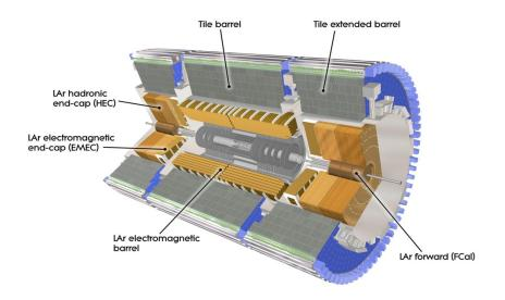
Figure 3.7: Schematic of the ATLAS calorimeter system. From [147].
