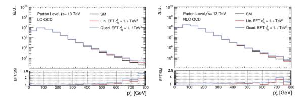
Figure 7.9: Parton level distributions of SMEFT predictions at LO (left) and NLO (right) QCD comparing the inclusion of the linear  $\Lambda^{-2}$  EFT order only(Lin. EFT) and with the inclusion of both the linear  $\Lambda^2$  and quadratic  $\Lambda^{-4}$  EFT order(Quad. EFT) with the  $c_{tq}^8$  four-quark Wilson coefficient set to 1.
