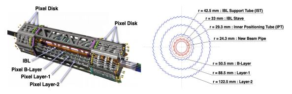
Figure 3.6: Schematic of the Pixel Detector including the IBL. From [140].
