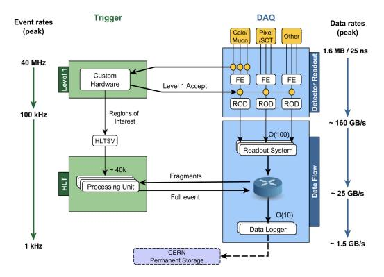
Figure 3.15: Schematic of the trigger and data acquisition system. From [163].
