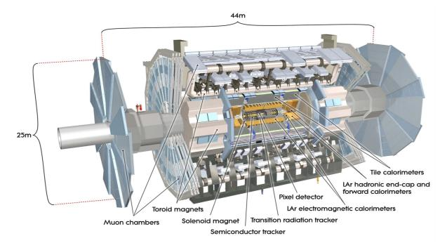
Figure 3.2: Schematic of the ATLAS detector. From [132].
