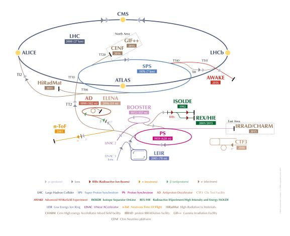
Figure 3.1: The CERN accelerator complex. From [131].
