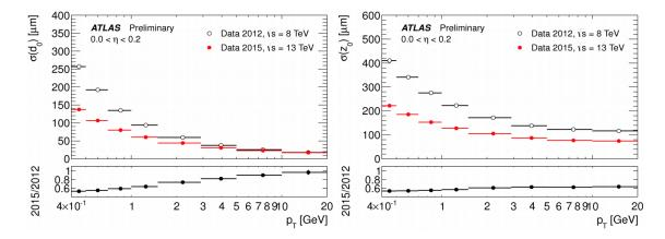
Figure 3.4: The resolutions of the track reconstruction parameters  $d_0$  (left) and  $z_0$  (right) as a function of the transverse momentum  $p_T$  with (Data 2015) and without the IBL (Data 2012). From [137].
