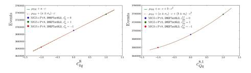
Figure 7.10: The particle level total rate predictions for various points in Wilson coefficient parameter space and the fitted function with the parameters evaluated at their best-fit and  $\pm \sigma$  value. The predictions are generated at LO QCD with the linear  $\Lambda^{-2}$  EFT order only (left) and NLO QCD with both the linear  $\Lambda^{-2}$  and quadratic  $\Lambda^{-4}$  EFT order included (right).
