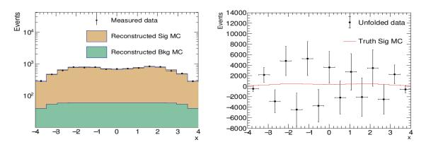
Figure 5.1: An example of how statistical fluctuations in the  $\boldsymbol{n}$ , an ill-conditioned response matrix R and an estimator  $\hat{\boldsymbol{\mu}}$  constructed with matrix inversion can result in large fluctuations in the estimator. The figure shows the measured data compared with the simulated Monte Carlo distributions on reconstructed level (Left) and the unfolded data and truth distributions (Right).
