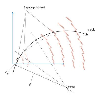
Figure 4.1: Sketch of a perfect helical track used to estimate the momentum  $p_T$  and transverse impact parameter  $d_0$  of a track seed. From [173].
