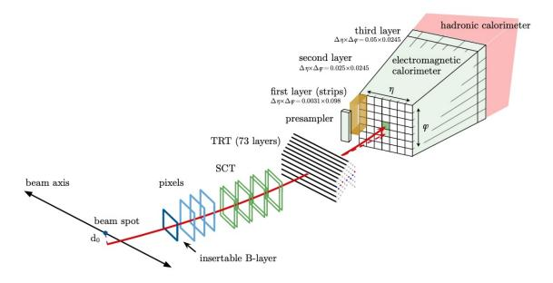
Figure 4.2: A schematic illustration of the path of an electron through the detector. From [177].
