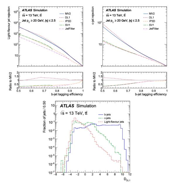
Figure 4.4: Light-flavour and c-jets rejection as a function of b-tagging efficiency for the DL1 algorithm compared with previous b-tagging algorithms (Top). Distribution of the output discriminant of the DL1 b-tagging algorithms for b-jets, c-jets and light-flavour jets on  $t\bar{t}$  simulated events (Bottom). From [187].
