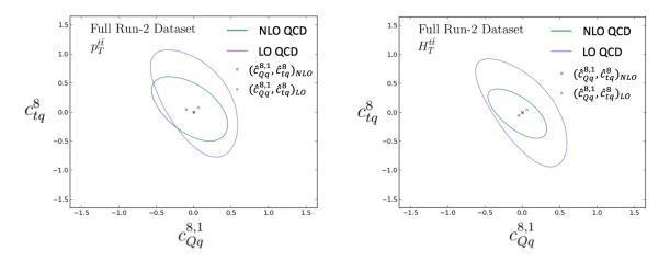
Figure 7.18: The confidence regions at a confidence level of 95% for the  $c_{tq}^8$  and  $c_{Qq}^{8,1}$ Wilson coefficients. The likelihoods were evaluated with the  $p_T^{t\bar{t}}(\text{Left})$  and  $H_T^{t\bar{t}}(\text{Right})$ unfolded distributions and covariance estimates using the matrix inversion method and the Full Run-2 dataset. The parameterization of the likelihood is constructed with the quadratic regression to either LO or NLO QCD SMEFT predictions.
