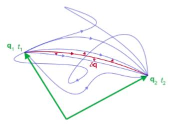
Figure 2.2: Different paths through configuration space. The red line indicates the path for which  $\delta S = 0$ . From [14].
