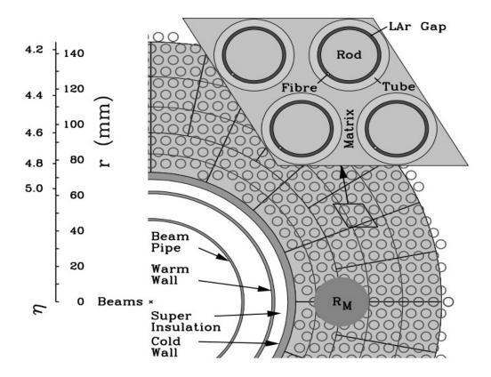
Figure 3.10: Sketch of the cross section of the FCAL. From [146].
