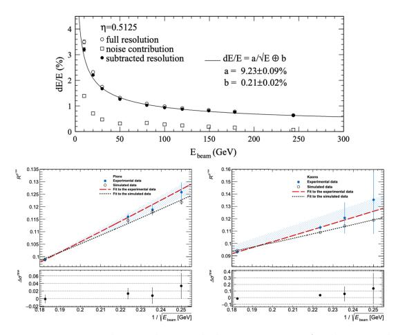
Figure 3.8: Energy resolutions relative to the beam energy  $E_{\text{beam}}$  for electrons in the LAr barrel ECAL (Top) and for pions (Bottom left) and kaons (Bottom right) in the Tile calorimeter. For the bottom plots the variables  $R^{\sigma^{\text{raw}}} = \frac{\sigma}{E_{\text{beam}}}$  and  $\Delta \sigma^{\text{raw}} = \frac{\sigma}{\sigma_{\text{MC}}} - 1$  are defined. From [148, 149].
