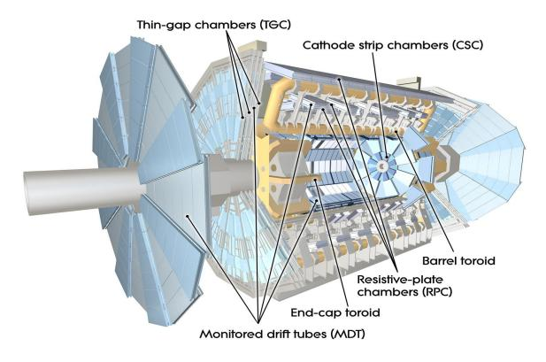
Figure 3.12: Schematic of the Muon spectrometer. From [132].
