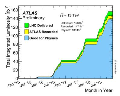
Figure 3.3: Total integrated luminosity of pp collisions at a center-of-mass energy of  $\sqrt{s} = 13$  TeV during the 2015 to 2018 data taking period. From [133].
