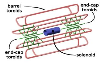
Figure 3.14: Schematic of the magnet system of the ATLAS detector. From [156].
