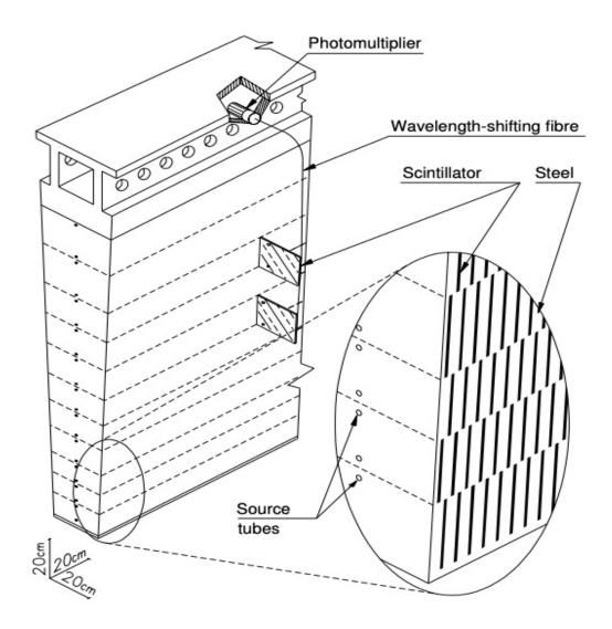
Figure 3.11: Sketch of a barrel wedge of the Tile Calorimeter. From [153].
