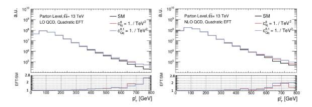
Figure 7.7: Parton level distributions of SMEFT predictions at LO (left) and NLO (right) QCD including both the linear  $\Lambda^{-2}$  and quadratic  $\Lambda^{-4}$  EFT order with the  $c_{tq}^8$  and  $c_{Qq}^{8,1}$  four-quark Wilson coefficients set to 1.
