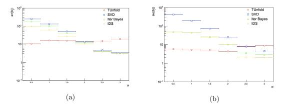
Figure 5.8: The bin-averaged bias for the unfolded distributions for varying  $\alpha$  for the TUnfold, SVD, Bayes and IDS method. The regularization parameters are chosen such that they a) unconditionally minimize the MSE and b) conditionally minimize the MSE with a minimal coverage of  $0.683 - \epsilon$  with  $\epsilon = 0.01$ . From [215].
