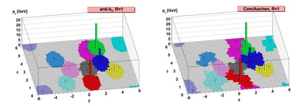
Figure 4.3: An illustration of calorimeter cells clustered with the anti- $k_t$  (Left) and Cambridge-Aachen (Right) algorithm for R = 1.0. The inputs come from a Monte Carlo event generated with Herwig. From [183].
