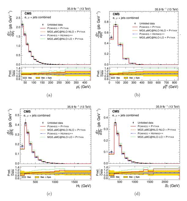
Figure 6.17: Unfolded distributions from a  $t\bar{t}$  differential cross section measurement in the l+jets decay channel measured at the CMS detector. Differential cross sections are shown as a function of the  $p_T$  of the lepton coming from the top quark  $(p_T^l)$ , the  $p_T$  of the leptonically decaying W boson coming from the top quark  $(p_T^W)$ , the scalar sum of the  $p_T$  of all jets  $(H_T)$  and the scalar sum of the  $p_T$  of all particles  $(S_T)$ . From [242].
