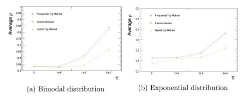
Figure 5.23: Average global correlation coefficient for a) the bimodal and b) the exponential distribution for all covariance estimation methods and various regularization strengths  $\tau$
