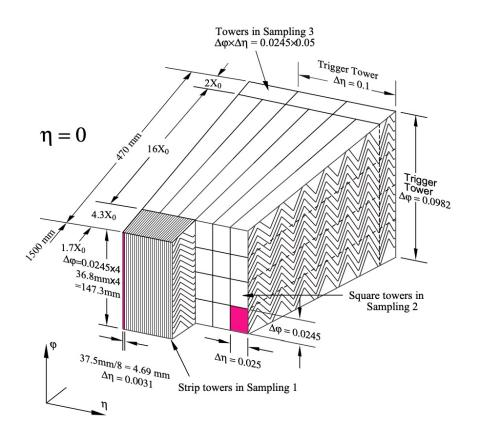
Figure 3.9: Sketch of the accordion structure of the EM calorimeter. The depths are expressed in both millimeters (mm) and material radiation length  $(X_0)$ . From [145].
