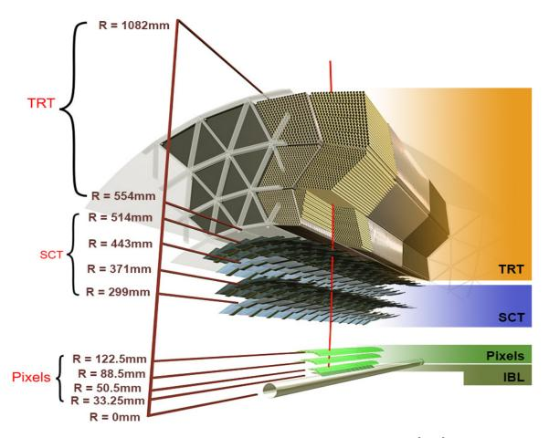
Figure 3.5: Schematic of the Inner Detector. From [132].
