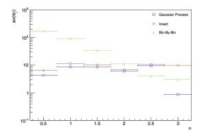
Figure 5.9: The bin-averaged bias for the unfolded distributions for varying  $\alpha$  for the Gaussian Processes, matrix inversion and bin-by-bin method. From [215].
