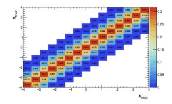
Figure 5.2: An example of an ill-conditioned response matrix as a result of detector smearing. This response matrix is estimated using simulated Monte Carlo events.
