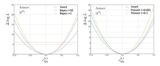
Figure 7.14: The log-likelihood difference  $\Delta \log L$  with  $L_{\max}$  maximized w.r.t. the  $c_{tq}^8$  and  $c_{Qq}^{8,1}$  Wilson coefficients simultaneously. The  $\Delta \log L$  is scanned for values of  $c_{Qq}^{8,1}$  with  $c_{tq}^8$  kept at its maximum-likelihood estimate. The likelihoods were evaluated with Asimov  $|y^{t\bar{t}}|$  unfolded distributions and covariance estimates for various amounts of regularization.
