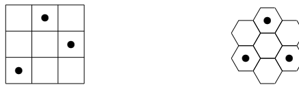
Figure 7.15: The 3 \times 3 Costas array and the corresponding A_{r,1} class of the honeycomb arrays.
