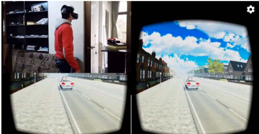
Figure 6. 2 Prototype one testing [Prototype one involved having to walk towards the motion sensor (Microsoft Kinect) to cross the road / avoid vehicles in a virtual environment. We used internal (VR environment) and external cameras to capture this video].
