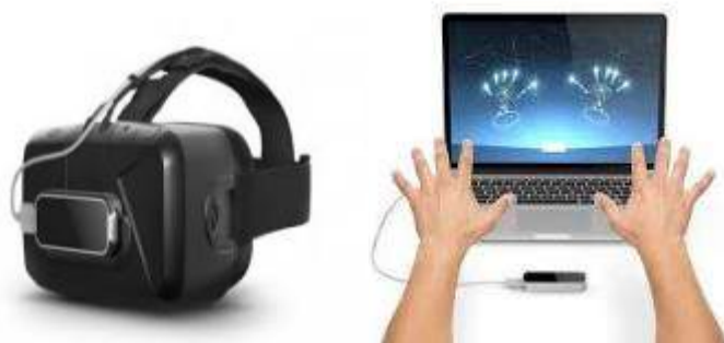
Figure 6. 9 Leap Motion sensor connected to VR headset /laptop to hand gestures
