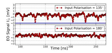
Figure 6.11: The train of signals disappears when the input polarisation is at 180°.
