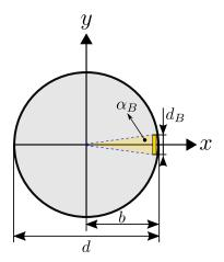
Figure D.1: Diagram illustrating the coverage angle  $\alpha_B$  for a traditional button pickup.
