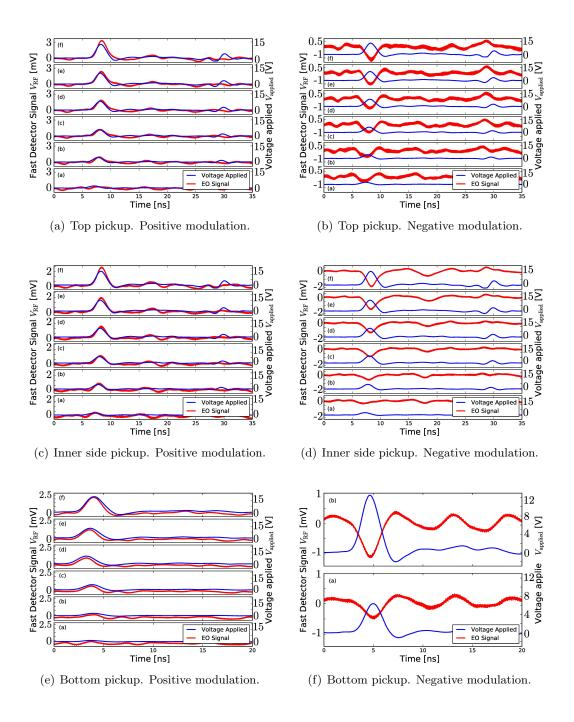
Figure 5.21: Averaged EO modulation when a fast voltage signal is applied on the electrodes of pickup one. The data recorded for Figure (f) only covered to 20 ns scope.
