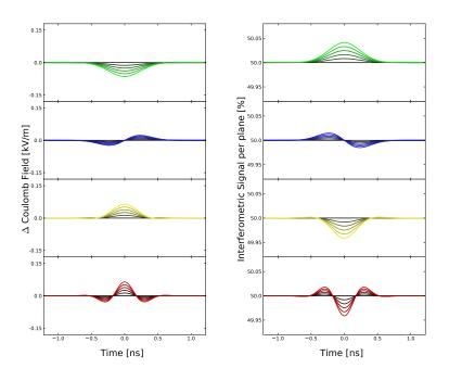
(a)  $\Delta$  Modulating field (Left - Right).(b) Interferometric signal combined from two pickups in the same plane.
