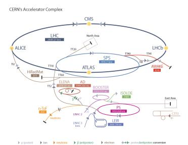
Figure 1.1: CERN accelerators chain [6].
