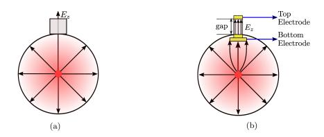
Figure 3.8: Concept designs for (a) the EO pickup with no electrode and (b) with electrode.
