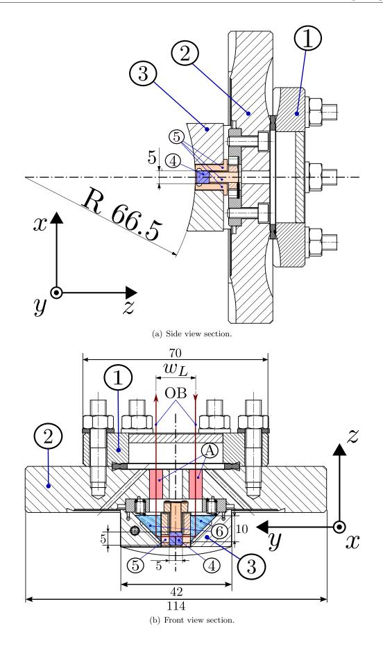
Figure 4.4: Technical drawings of pickup zero (all the units are in millimetres) [54].
