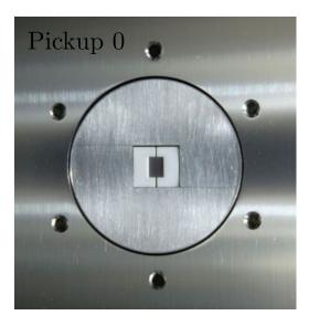
Figure 4.12: Button zero from inside the pipe.
