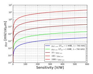
Figure 7.3: Isogradient curve for  $g_{\rm RF} = 1 \,{\rm mV}/100 \mu{\rm m}$  at 780 nm, with  $P_{sat} = 1 \,{\rm mW}$ .
