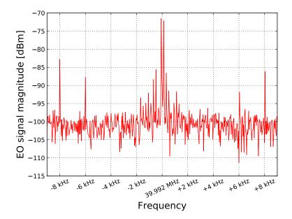
Figure 6.21: Frequency spectrum of the EO pickup signal around the  $922^{nd}$  harmonic of the SPS revolution frequency.
