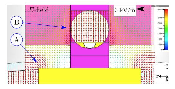
Figure 4.20: Vector field map produced by CST over the crystal section XZ at y = 0 for pickup one. The instant corresponds to the peak field at  $r_0 = 68.5$  mm. The field goes through a shorter path A towards the grounded pipe and through B due to the lower dielectric constant of Macor.
