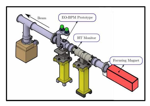
Figure 1.5: Representation of the section of the SPS ring where the EO-BPM was installed.
