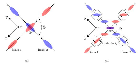
Figure 1.2: Diagrams of the current collision geometry (a), and the crab cavity mechanism (b): the bunch is rotated before the Interaction Point IP to orient the bunches head-on and is kicked back to the original position afterwards.
