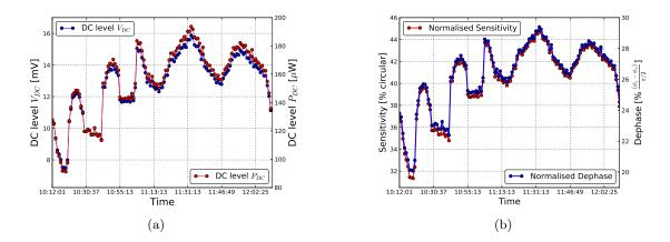
within a range from 31% to 45%, whereas the DC level that determines the contrast in 6.14(a) more than doubles, from about 7 mV up to 16.5 mV:
