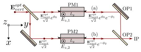
Figure 2.9: Mach-Zehnder interferometer with two LNB crystals (PM1 and PM2) acting as phase modulators placed in each of the two equally long arms.
