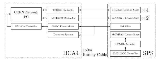
Figure 5.4: Flux diagram of the control instrumentation.
