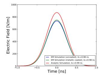
Figure 4.17: Coulomb field time-profile curve inside the LNB sample for pickup zero  $(r_0 = 68.0 \text{ mm})$ .
