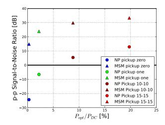
Figure 7.2:  $\rm SNR_{p-p}$  comparison between the prototype acquisition system (NP) and MSM detector.
