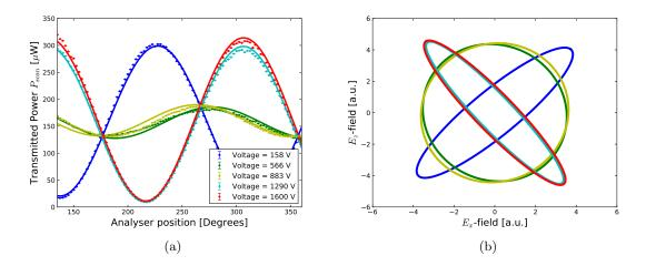
Figure 2.16: Experimental polarisation scans from 135° (points) and fits (continuous curve) (a) of the different polarisation states (b).
