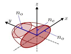
Figure 2.1: Section of the index ellipsoid on the y-cut (shaded) plane when the optical beam is propagating along the y axis. The ellipsoid axes are shown in blue:  $n_o$  is the refractive index along x and y, and  $n_e$  along z.
