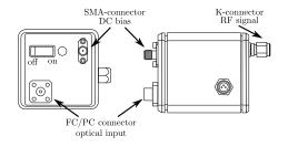
Figure 5.10: Technical drawing of the fast detector.
