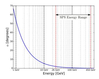
Figure 3.4: The angle  $\alpha$  subtended by the bunch Coulomb field as a function of proton energy. The SPS energy range covers from injection at 26 GeV up to 450 GeV.
