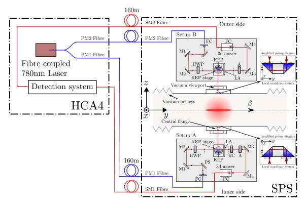
Figure 5.1: Layout of the optical setup for the EO-BPM experiment.
