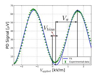
Figure 2.14: Experimental transfer function for a 10 mm long and 5 mm thick LNB sample.
