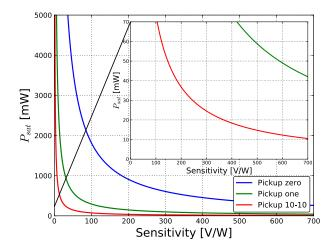
Figure 7.4: Isogradient curves for  $g_{\rm RF} = 1 \, {\rm mV}/100 \, \mu {\rm m}$  at 780 nm.
