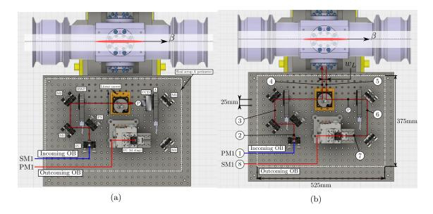
Figure 5.3: Example of the OB trajectory when the knife-edge prism is retracted (a) and placed in the final position (b) for setup A.
