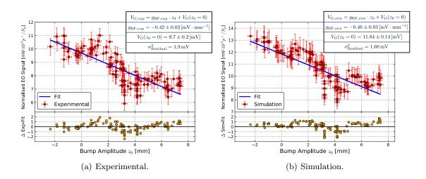
Figure 6.16: Experimental EO modulation peak  $V_G$  (a) compared to the expected simulation (b).
