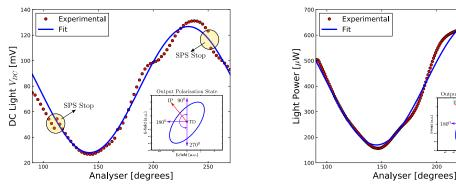
(a) Photodiode DC level scan during acquisition.
