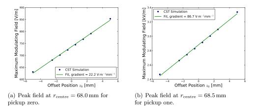
Figure 4.34: Field strength peak gradient in the crystal as a function of the beam offset  $z_0$  according to the CST simulations.
