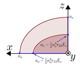
Figure 2.2: The index ellipsoid section with E = 0 occupies more surface (clearer) than when  $E \neq 0$  (darker).
