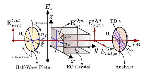
Figure 2.5: Amplitude modulation diagram.
