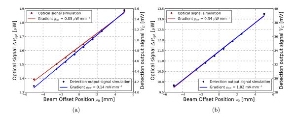
Figure 5.18: Gradients of the optical signal  $g_{opt}$  and the output detection system  $g_G$  as a function of the position for (a) pickup zero and (b) pickup one when the output polarisation estate is circular ( $\Gamma_0 = \pi/2$ ).
