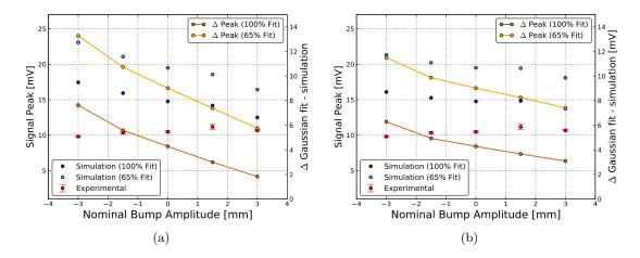
Figure 6.24: (a) Experimental and simulated signal maximum as a function of the bump amplitude, and the difference between them both for the perfect Gaussian fit (100%) and the 65% reduction in bunch length; (b) Peak signal scaled accordingly assuming a constant bunch length of 2.88 ns.
