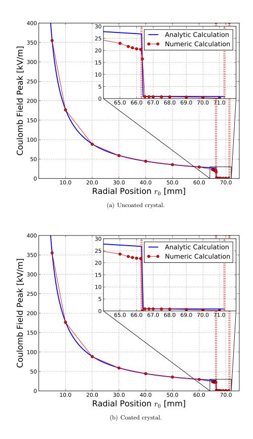
Figure 4.15: Numerical electromagnetic and analytic simulations of the peak Coulomb field along the radial transverse position  $r_0$  over the pipe section for pickup zero.
