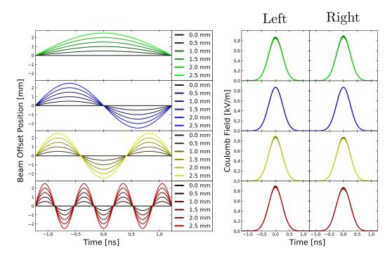
(a) Representation of the HT instabilities of modes 0,(b) Modulating field inside a LNB crystal located 1, 2 and 6. at 30 mm from the beam.
