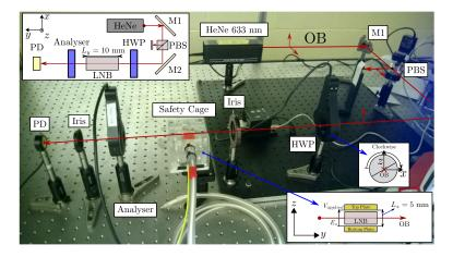
Figure 2.13: Experimental electro-optic characterisation setup.
