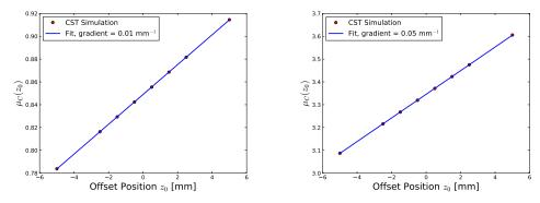
(a)  $\mu_C(z_0)$  at  $r_{\text{centre}} = 68.0 \text{ mm}$  for pickup zero. (b)  $\mu_C(z_0)$  at  $r_{\text{centre}} = 68.5 \text{ mm}$  for pickup one.
