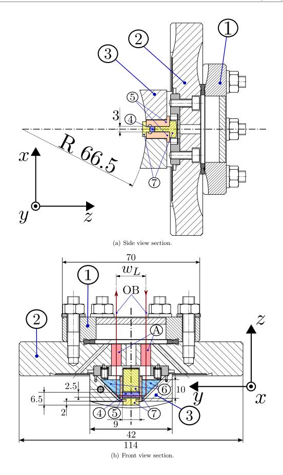
Figure 4.5: Technical drawings for pickup one (all the units are in millimetres) [55].
