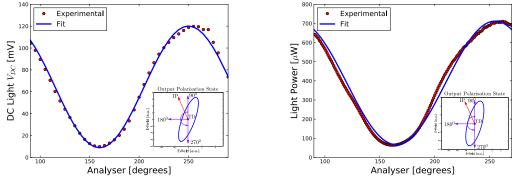
(a) Photodiode DC level scan during acquisition.
