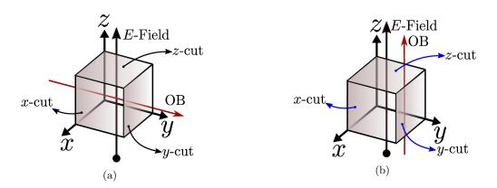
Figure 2.3: (a) Transverse modulation and (b) Longitudinal modulation geometries.
