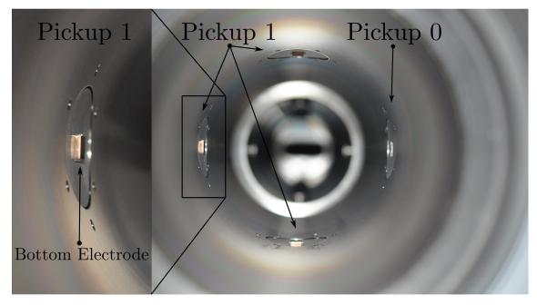
Figure 4.13: Buttons one and zero from inside the pipe.
