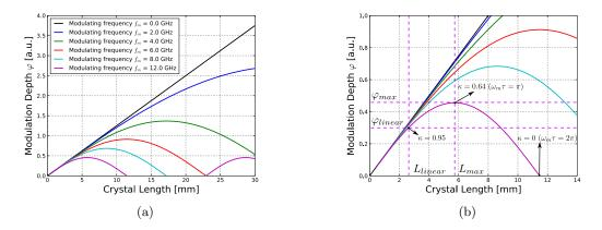
Figure 2.20: (a) Modulation depth against crystal length for the extraordinary refractive index  $n_e$ ; (b) zoomed in amplification until 14 mm with labels to mark the linear and maximum modulation regimes for the case  $f_m = 12 \text{ GHz}$ .
