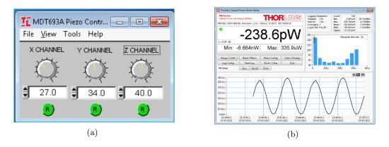
Figure 5.5: 3-axis panel control (a) and readout interface of the power meter software (b).
