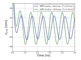
Figure 4.25: Resonances of the rigid mode for a pickup one installed in the LHC (30 mm) and the SPS (66.5 mm).
