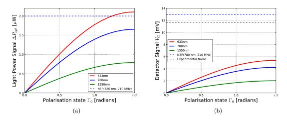
Figure 5.16: Optical power signal  $\Delta P_{opt}$  (a) and detection signal voltage (b) as a function of the output polarisation, for the 5 mm cubic crystal in pickup zero modulated by 750 V/m electric field that corresponds to the SPS nominal bunch. The NEP at 780 nm and the experimental noise are also calculated.
