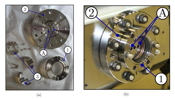
Figure 4.3: (a) Button pieces, central flange and viewport; (b) EO pickup mounted in the horizontal plane of the SPS pipe.
