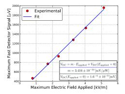
Figure 5.23: Maximum EO signal as a function of the field applied resulted from the characterisation of the inner side EO pickup one for positive signals.
