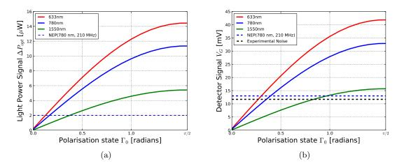
Figure 5.17: Optical power signal  $\Delta P_{opt}$  (a) and detection signal voltage (b) as a function of the output polarisation, for the 9 mm long crystal in pickup one modulated by 2.86 kV/m electric field that corresponds to the SPS nominal bunch. The NEP at 780 nm and the experimental noise are also calculated.
