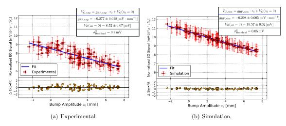
Figure 6.17: Experimental EO modulation peak  $V_G$  (a) compared to the expected simulation (b) when the sensitivity drift has been removed.
