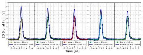
(a) Experimental measurements for each nominal bump amplitude in comparison with the prediction when assuming the bunch length obtained directly from the signal fit.
