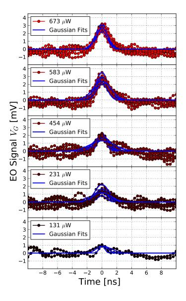
Figure 6.8: Experimental signal at different laser input power values with the baseline substracted.
