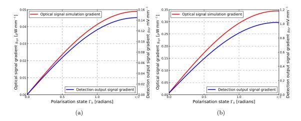
Figure 5.19: Gradients of the optical signal  $g_{opt}$  and the output detection system  $g_G$  as a function of the polarisation estate  $\Gamma_0$  for pickup variants zero (a) and one (b).
