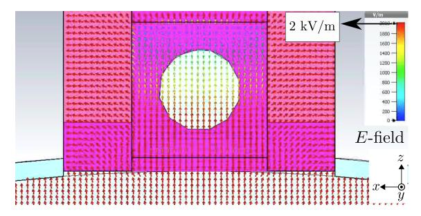
Figure 4.16: Vector field map produced by CST over the crystal section XZ at y = 0 for pickup zero. The instant corresponds to the peak field at  $r_0 = 68.0$  mm.
