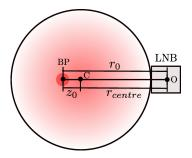
Figure 4.32: Diagram with the main geometrical parameters in the gradient calculation: BP is the beam position; C is the centre of the pipe; O is the crystal position.
