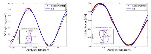
(a) Photodiode DC level scan during acquisition.
