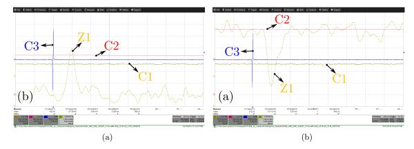
Figure 6.3: Example of the oscilloscope display appearance for a negative (a) and a positive (b) bunch-induced EO signal.
