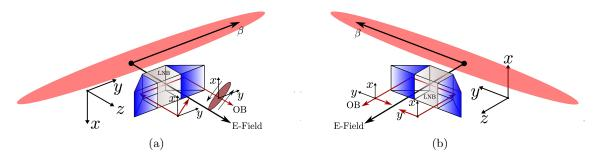
Figure 3.9: Conceptual designs for (a) a crossed polarisers pickup and (b) a phase modulator pickup.
