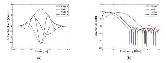
Figure 1.3: Typical HT signals for modes 0, 1, 2, and 6 in the time-domain (a) and the corresponding frequency bandwidth (b).
