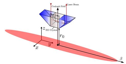
Figure 3.7: Interaction between the Coulomb field of the passing bunch and the conceptual EO pickup.
