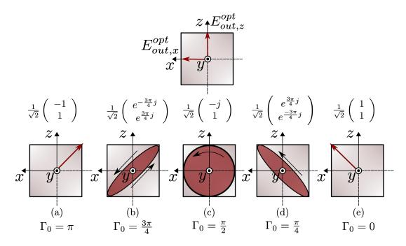
Figure 2.6: Crystal output face with some relevant polarisation states associated with the vector  $\mathbf{E}_{out}^{opt}$ : linear anti-phase parallel to the analyser ( $\Gamma_0 = \pi$ ), circular ( $\Gamma_0 = \frac{\pi}{2}$ ), in-phase perpendicular to the analyser ( $\Gamma_0 = \frac{\pi}{4}$ ) and two half-way elliptical states ( $\Gamma_0 = \frac{3\pi}{4}$  and  $\Gamma_0 = \frac{\pi}{4}$ ).
