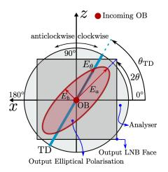
Figure 2.15: Polarisation scan mechanism represented from the crystal output face view. Angles  $\theta_{TD}$  and  $2\theta$  determine the directions of the transmission direction of the analyser and the input polarisation, respectively.
