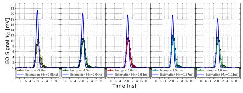
(b) Experimental measurements for each nominal bump amplitude in comparison with the prediction when the bunch length is shortened by 65% with respect the signal fit.
