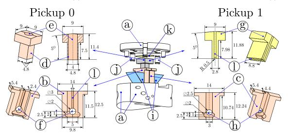
Figure 4.8: Assembly drawing of the ceramic holder and the button [56, 57].
