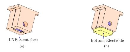
Figure 4.9: Depiction of the crystal sample embedded in the ceramic holder for pickup zero (a), and the bottom electrode for pickup one (b).
