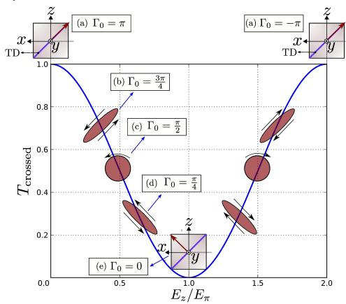
Figure 2.7: Transfer function (eqn. 2.28) with the associated output polarisation states after the crystal also depicted in Figure 2.6.
