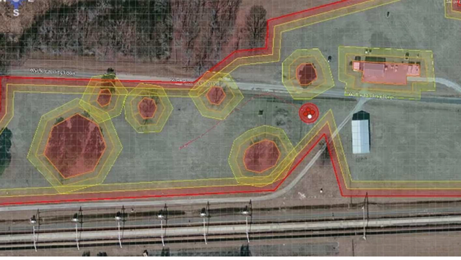
Fig. 1: Dual geofencing used by Safeguard [11], showing NFZ (red), termination (orange) and warning areas (yellow).
