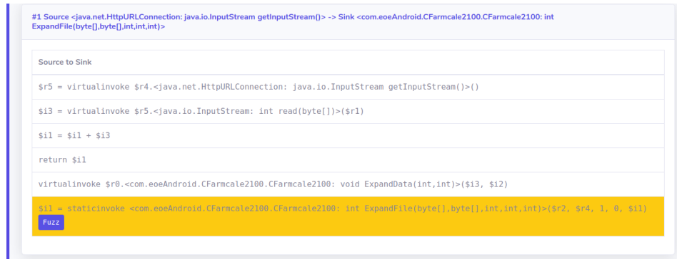
Figure 5.4: Flow View . An analyst can visualize a taint analysis and select native flow to fuzz.
