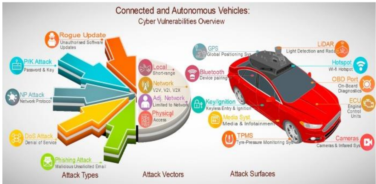
Figure 12: An overview of attack types, vectors and surfaces of an AV [50]
