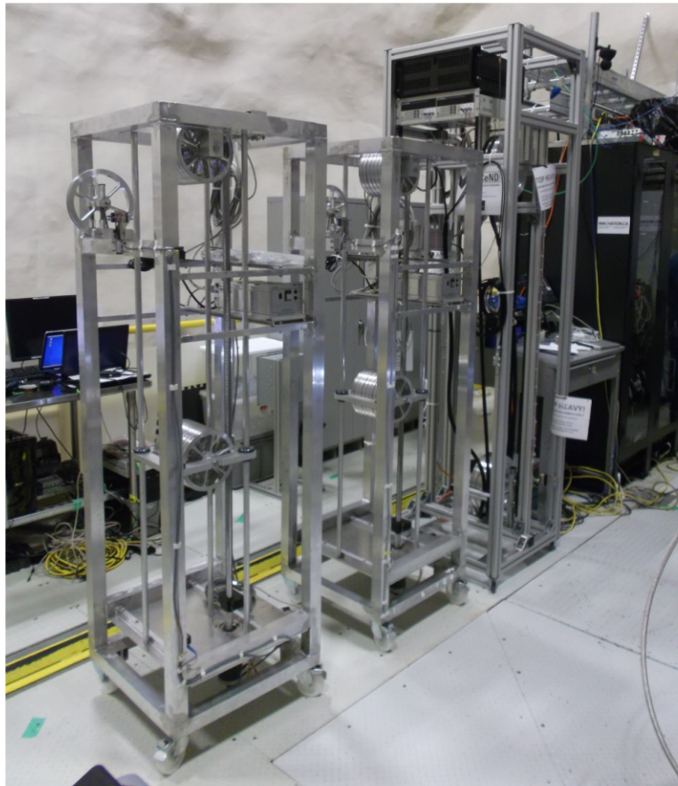
Figure 2.32: Picture of the gamma calibration deployment system for Cal F tube (two racks on the left) and neutron calibration deployment system (taller rack on the right).
