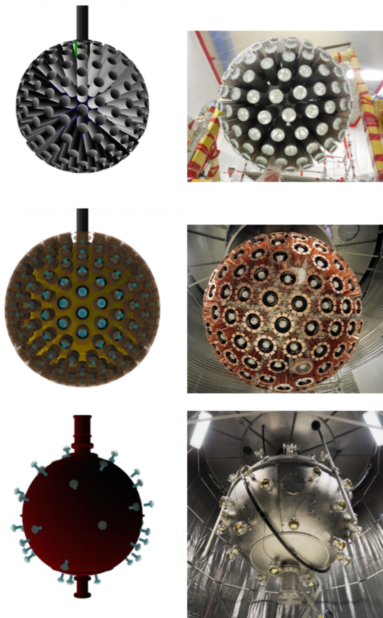
Figure 5.1: Ray traced simulated detector components compared to real DEAP-3600 detector components. Top: Acrylic vessel with light guides attached. Middle: copper heat shorts. Bottom: Steel shell and veto PMTs [61].
