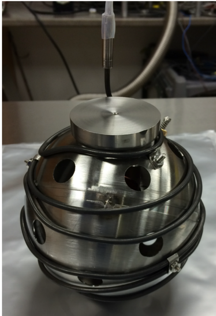
Figure 2.14: Image of the TPB evaporation source. The black filament is a coil heater that by heating the crucible inside the sphere allow the evaporation of the TPB powder for deposition [56].
