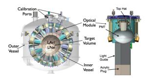
Fig. 2: The MiniCLEAN detector and the optical modules.
