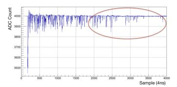
Fig. 3: Raw waveform of a scintillation event. The region circled is dominated by single photon pulses.
