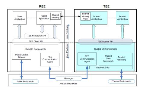
Fig. 1. GlobalPlatform TEE system architecture [22].
