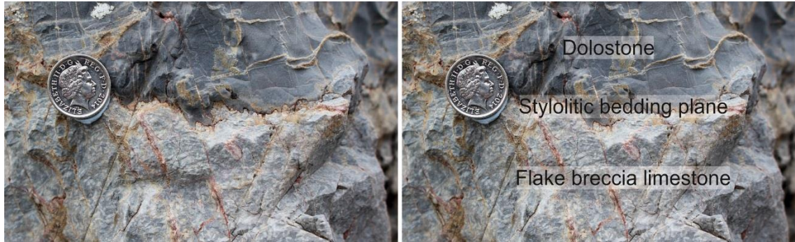
Figure 5.2: Flake breccia limestone bed alternating with massive dolostone; about 5 m below the contact between PAT and Lossit Formations.
