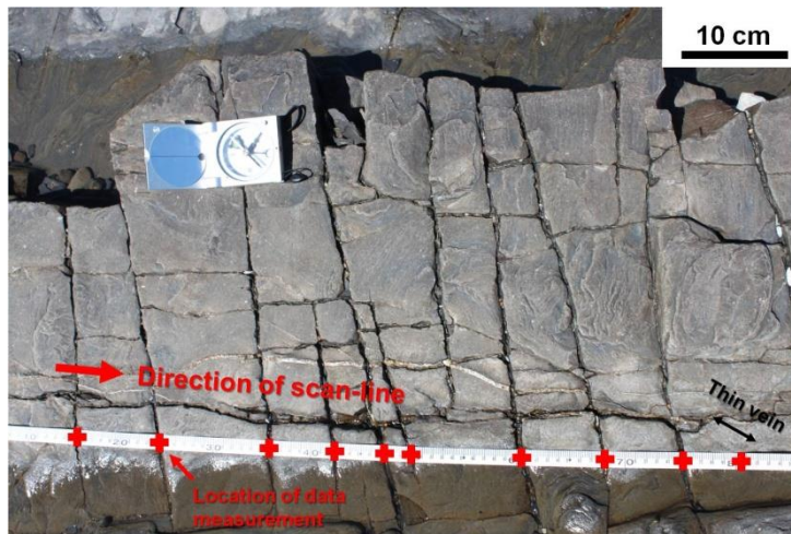
Figure 3.4 Fractures measured along a scan-line. All fractures and veins traversing the tape measure were analysed.
