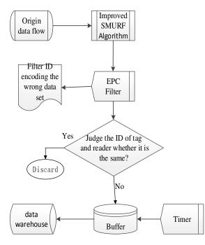
Fig.1 Framework of RFID redundant data cleaning
