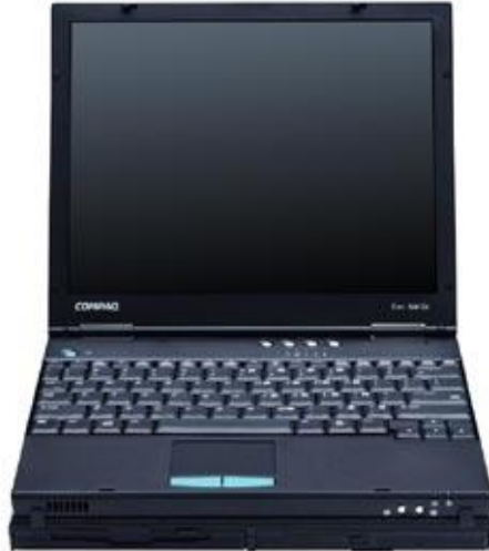
Figure 1.2: Machine and Chipset 2. The HP Compac Evo N410c, endowed with Intel Pentium III processor, has the SMRAMC register unlocked and SMRAM opened after the bootup process.
