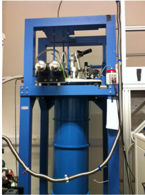
Figure 6.5.: Oxford Instruments Triton 200 dry dilution refrigerator. Already installed coaxial lines, well controlled bath temperature from as low as 10mK, and a programmable 12T magnet made it well suited to weak localisation studies.
