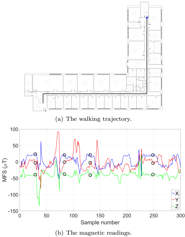
Figure 4 The magnitude of each of the three axes measured from a single walk through non-repeated positions on the ground floor of the test bed. The black circle pinpoints the positions with a similar reading.
