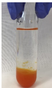
Figure 11. Ultra-Clear™ centrifuge tube containing a tomato subchromoplast compartment suspension in sucrose gradient before centrifugation
