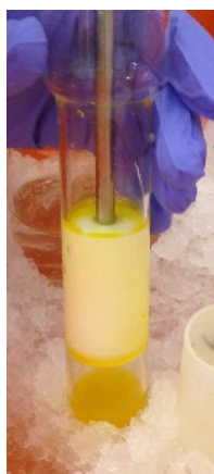
Figure 10. Homogenisation of the pepper chromoplast juice using a potter-Elvehjem tissue grinder
