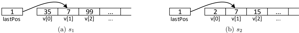
Figure 1: Two shared states satisfying the same base condition \Phi_3 : lastPos = 1 \wedge v[1] = 7 .
